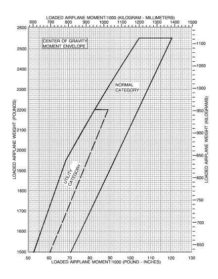
Figure 6-7. Center of Gravity Moment Envelope
