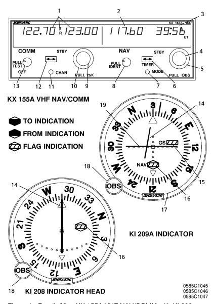
Figure 1. Bendix/King KX 155A VHF NAV/COMM with KI 208 or KI 209A Indicator Head (Sheet 1 of 7)
