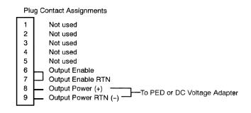
Figure 3. Mating Plug Wiring
