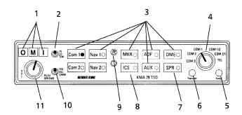
1. MARKER BEACON ANNUNCIATOR LIGHTS -- The three-light marker beacon receiver built into the KMA 28 gives a visual and aural signal when the ship's antenna passes over a 75 MHz beacon. The blue, amber, and white lights on the faceplate, as well as the audio tones, identify the beacon type.
