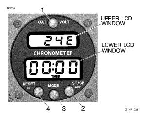
Figure 1. Astrotech Model TC-2 Clock/OAT/Volt Indicator
