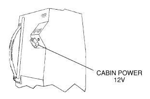
Figure 1. 12 Volt Cabin Power System Connector
